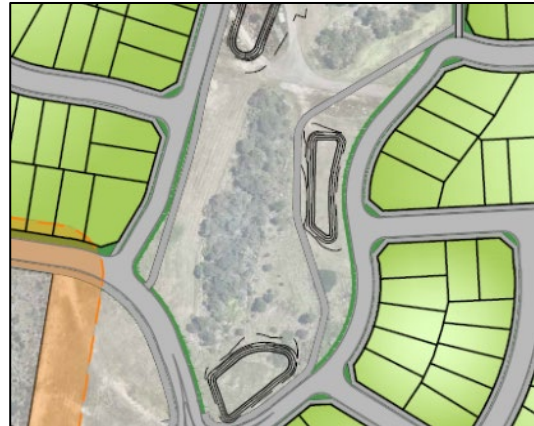
Plate 19: Revised designs depicting road design moved south to avoid PCT 4059
